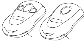
Figure MA-3 Pry case open at the notch
